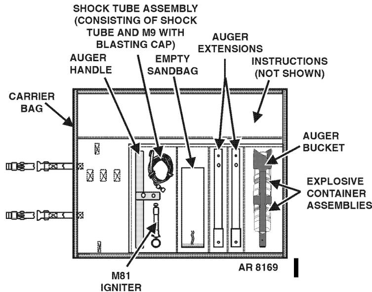
Demolition Kit, Blasting: Fighting Position Excavator, M300.
