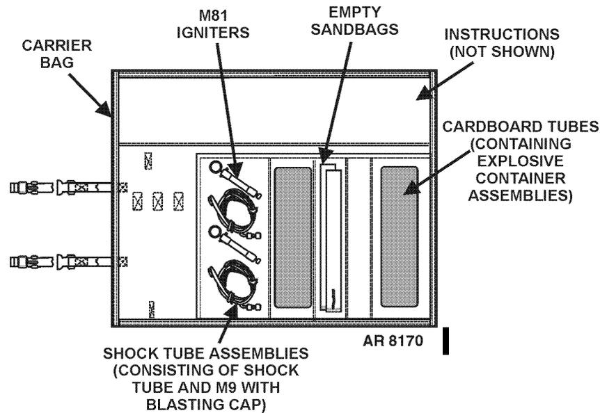
Demolition Kit, Blasting: Fighting Position Excavator, Reload Kit, M301.
